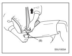
To unfasten the belt, push the red button on the buckle (B) and allow the belt to retract.
